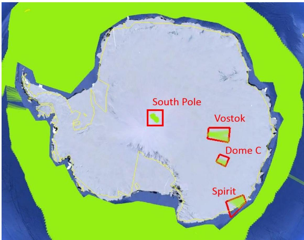
**Figure 12. Overview of CryoSat-2 tracks acquired in SAR mode that will be utilised in this study. Most data, in accordance with the operational mask, is acquired offshore, but inland there have been several dedicated SAR acquisitions at our identified study sites.**
