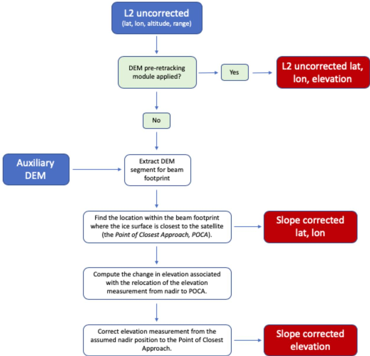
Figure 9. Block diagram showing the input data, processing steps, and output fields for the echo relocation. Blue blocks indicate input data, green blocks indicate decisions, white blocks indicate processing steps, and red blocks indicate output fields. Full details of the method are given in Roemer *et al.* (2007).
