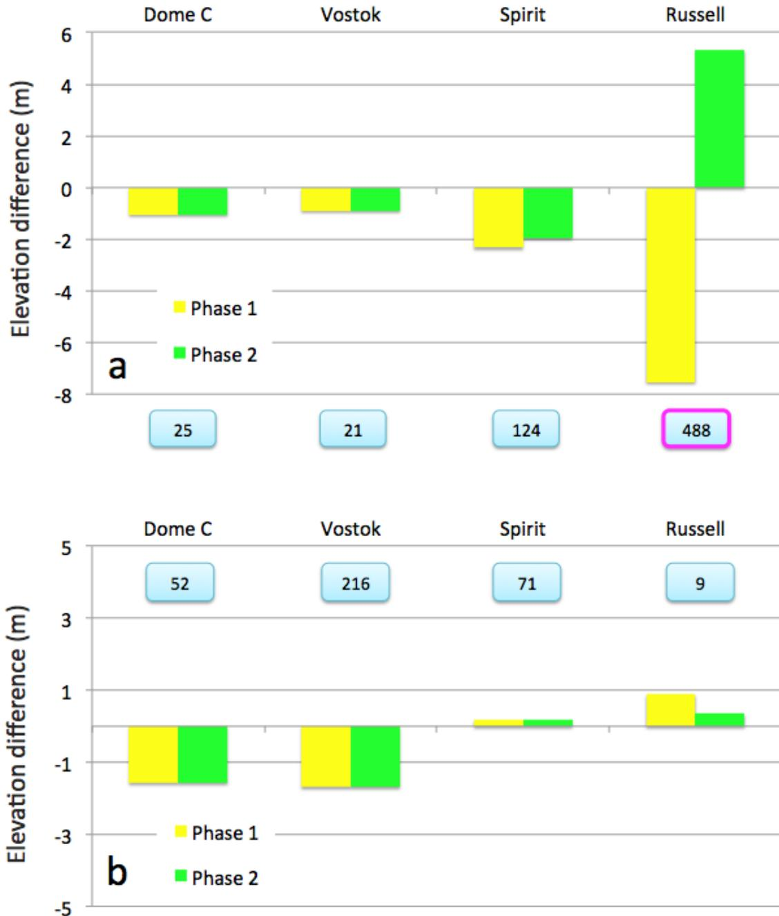
Figure 7. Elevation biases of ESA, SPICE Phase 1 and SPICE Phase 2 pLRM data, relative to (a) IceBridge and (b) ICESat reference datasets. The cyan boxes indicate the number of validation pairs at each site, which were used in the inter-comparison. Boxes highlighted in magenta indicate a significant difference between Phase 1 and Phase 2 datasets, based on a 5% significance threshold. No ESA data are present because generation of pLRM does not form part of the current CryoSat-2 ground segment.
